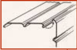
Pinch-Proof Section Joint: Strong design eliminates problem with other designs of joints. Joint Built Into Sectional Steel Garage Door.
