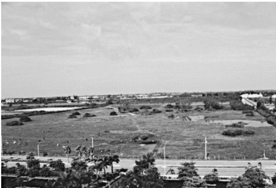
Exposure C Example (Source: ASCE 7-10)
