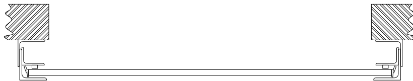
Figure 3 No Wind Load With Windlocks
