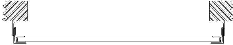
Figure 1 No Wind Load No Windlocks
