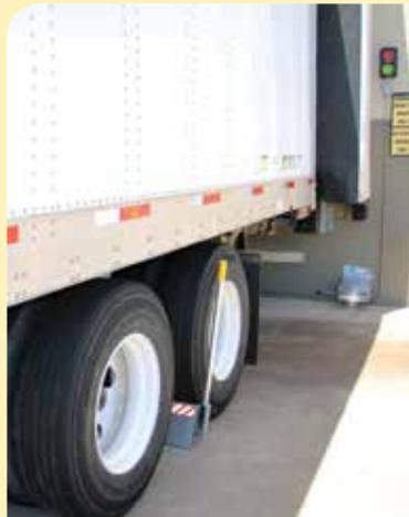
The Versachock is a vehicle restraint system that accommodates a variety of
