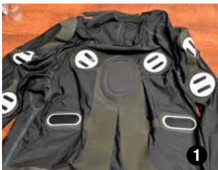
SENSOR SUIT: These three photos show (1) the sensors inside the bodysuit and (2) the exterior front and (3) exterior back.
