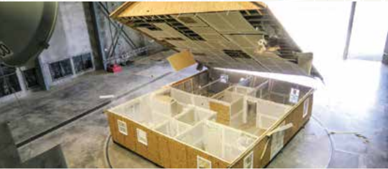
For maximum protection from severe weather, Fortified Gold requires a continuous load path.
