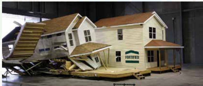
A high wind demonstration at the IBHS Research Center shows the importance of a continuous load path, a Fortified Gold designation requirement.
