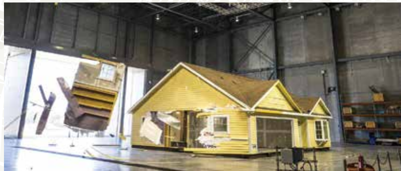
Tests at the IBHS Research Center show cascading damage that can result from garage door failure.
