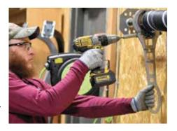
The tool eliminates the need for winding bars and reduces the time needed to wind springs. Other benefits of spring-winding tools are featured on pp. 58-62. www.surewinder.com
